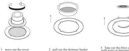
3 Take out the filter core then clean with water or detergen  $_{\circ}$
