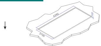
The location where to place the swimming spa should be in sunken dug pit measure: 4390 mm  $\times 2700$  mm  $\times 100$  mm
