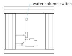
Open the skirt under the jet,the water  $\frac{\texttt{product}}{\texttt{duct}}$ column switch can adjust the heigh of the water column
