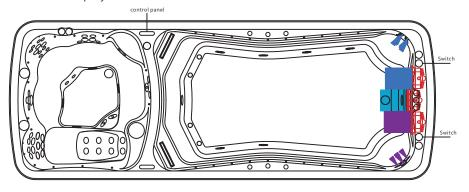
2. turn on the Surfing pumpl, 2, 3 by the panel, then spray water, adjust the switch to control the jets on the seat spray water
