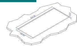
The location where to place the swimming spa should be in sunken dug pit measure: 6200mmx2600mmx100mm
