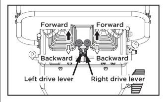
Pushing both drive control levers forward simultaneously, moves the excavator forward. Similarly, pulling both drive control levers backward simultaneously, moves the excavator backward. The front of the excavator is the direction where the dozer is present.
