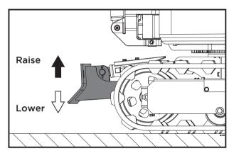
2. While undertaking earth moving work, control both drive levers with the left hand and the control lever for dozer with the right hand.
