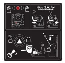
Hold the lever towards to right side to unlock the seat, then do adjustment.
