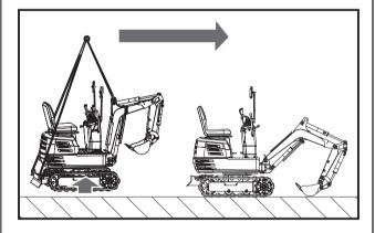
The excavator cannot travel on the muddy road with the slewing platform perpendicular to the tracks, so as to prevent the tracks from being involved in the mud.
