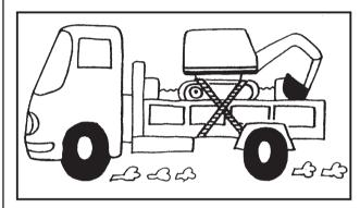
8. Before unloading, remove the swing lock pin and then raise the dozer and bucket from the truck bed.
