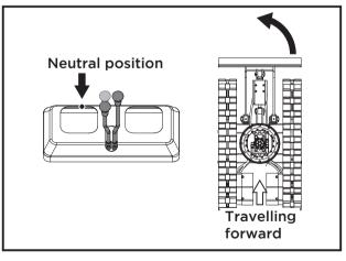
2. While travelling backward, push back the left drive lever into the neutral position, and keep pulling the right lever in the backward position, back of the excavator will turn to the right.
