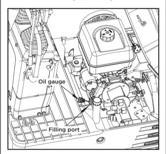
4. Let the engine idle for approx. 5 min. Check the engine oil level. To check the engine oil level, insert the oil gauge completely into the respective port opening and pull out again. If the oil level lies between both markings, no oil must be added.
