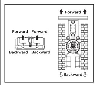
IMPORTANT If the crawler is clogged with sand or gravel while working on soft ground, lift up one crawler with the help of the boom, arm and bucket and let the crawler rotate to shake off the sand and gravel.
