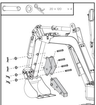
When the thumb is not in use, pull out the lower R-pin and the pin shaft, fold up the thumb into the bracket and fix it in the upper position with the previously pulled out parts.
