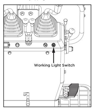
↑ IMPORTANT The ambient lighting of the machine must be above 500Lux.
