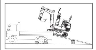
A DANGER When the excavator reaches the point between the ramps and the truck bed, halt and then move very slowly until the excavator reaches the horizontal position.
