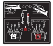
Pull back the black control lever to raise the dozer. Pushing the lever forward to lower the dozer.
