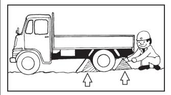
2. Use fixing plates to secure the ramp properly. Connect the ramps directly with the truck bed.
