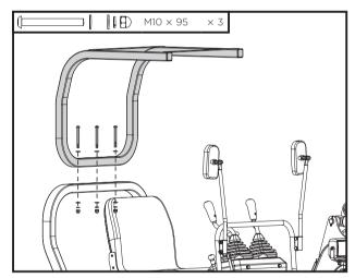
Align the holes in the canopy top with the holes in the upper frame of the canopy as shown. Fasten the canopy top in place with the provided M8x25 bolts, washers and nuts.
