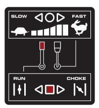
THROTTLE CONTROL The throttle control regulates the speed of the engine. The throttle control moves between Slow ... and Fast ... positions
