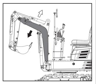
Men lowering the boom, make sure that it does not hit the dozer and that the bucket teeth do not touch the dozer.
