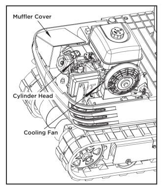
A IMPORTANT Cooling fan must be clean in order not to overheat the engine and allow free flow of air through the system.
