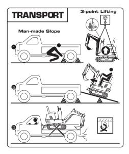
Using 3-point Lifting way or ramp to load or unload the excavator.
