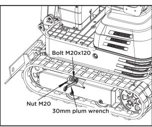
1. Tension the crawler in the lifted position, so that the distance (clearance between the track roller and the inside surface of the crawler) is 10 to 15 mm (see illustration), (In this case, the crawler seam is positioned on the top centre between the idler and the sprocket.
