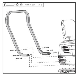
Align the holes in the upper frame with the holes in the lower frame of the canopy as shown. Secure the connection with the provided M10x95 bolts, washers and nuts.
