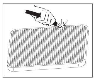
IMPORTANT If the air suction is still inadequate, or the colour of the exhaust gases is abnormal even after the cleaning, the air filter element must be replaced.
