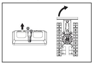
2. Pull the left drive lever backward, back of the excavator will turn to the right.
