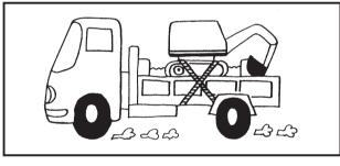
5. Do not brake abruptly with the excavator loaded. Fatal accidents could happen.
