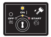
ENGINE ON/OFF/START SWITCH The engine switch has three positions. OFF - engine will not start or run. ON - engine will run. Start - engine will ignite
