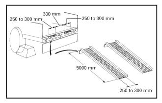
3. For additional safety, use blocks or struts under the ramps and the truck bed.
