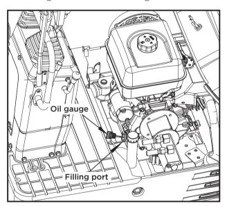
⚠ IMPORTANT Use engine oil with the correct viscosity. (according the outside temperature)
