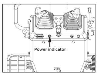
When the power indicator light is off, first check whether the fuse is blown. After the fuse is replaced, the fuse is normal, indicating that the battery is dead and needs to be charged; If the fuse is still blown after replacement, it is necessary to find professional maintenance personnel to repair the circuit.
